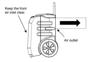
A maximum of 5m of 170mm ducting can be attached. Run the ducting straight and avoid bends and kinks.
